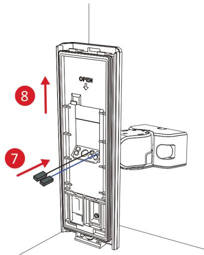
**9.** Remove the bracket tamper connector.
